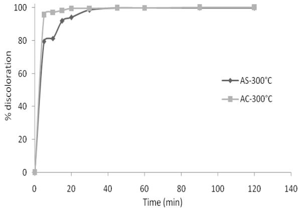
**Figure 4.** Effect of contact time on adsorption of methylene blue by AC-300°C and AS-300°C.
