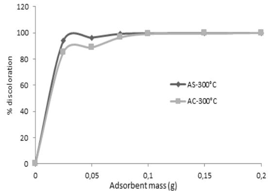
**Figure 6.** Effect of adsorbent mass on MB adsorption.
