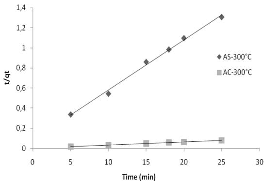
Figure 10. Pseudo-second order for the adsorption of the methylene blue on AS-300°C and AC-300°C
