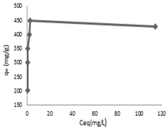
Figure 8. Adsorption isotherm of methylene blue onto AS-300°C
