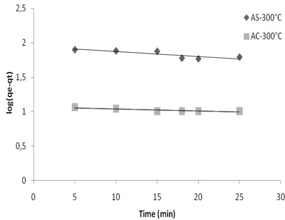
Figure 9. Pseudo-first order for the adsorption of the methylene blue on AS-300°C and AC-300°C
