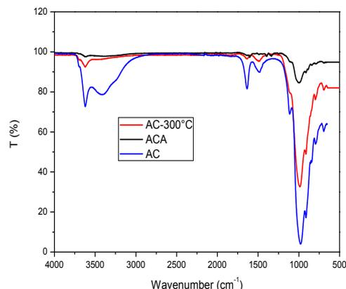
Figure 3. FTIR spectra of AC, AC-300°C and ACA.
