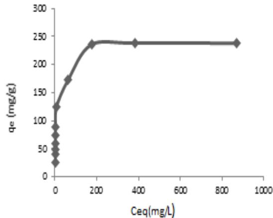
Figure 7. Adsorption isotherm of methylene blue onto AS-300°C
