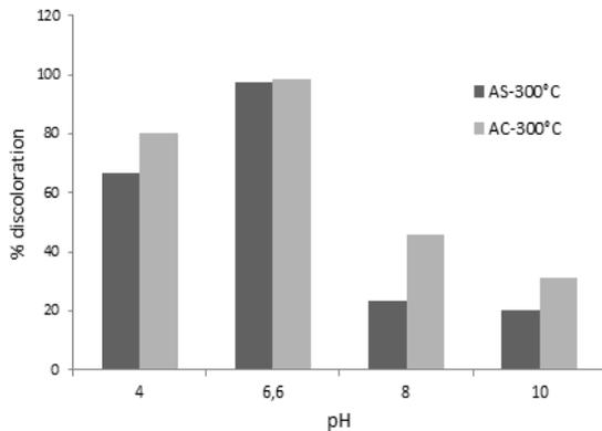
**Figure 5.** Effect of pH on adsorption of methylene blue by AC-300°C and AS-300°C.
