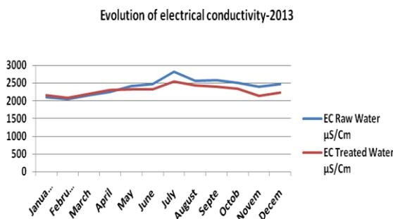
**Figure 2.** Graphic representation of the evolution of the EC at the inlet and at the outlet of the WWTP.
