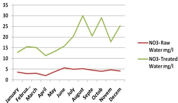
**Figure 4.** Graphic representation of the evolution of  $NO_3^-$  at the inlet and the outlet of the WWTP-2013
