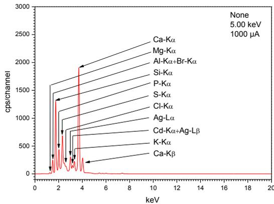
**Figure 4.** XRF spectrum of sludge of Guelma wastewater treatment plant achieved without a filter, 5.00 kV and 1000  $\mu$ A.
