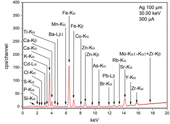
**Figure 1.** XRF spectrum of sludge of Guelma wastewater treatment plant achieved with a silver filter of 100 μm, 30.00 kV and 300 μA.
