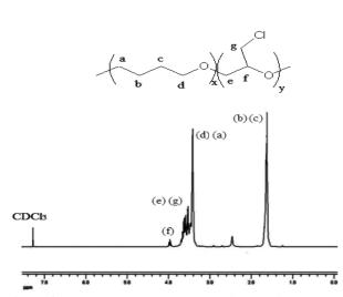
*Figure 2. H-NMR* (300 *MHz*) in CDCl3 of Poly (ECH-co-THF).
