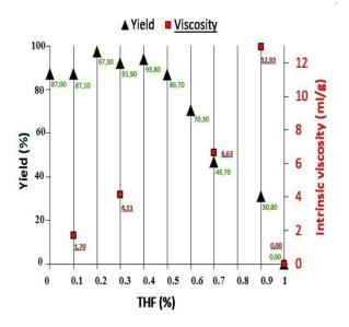
*Figure 7. Effects of the molar fraction of the monomers in the yield and intrinsic viscosity of the copolymerization.*
