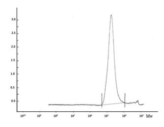
Figure 4. GPC curve of poly (ECH-co-THF) prepared with amounts Equimolar, 10% Maghnite-H+, T = 20 °C.
