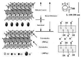
**Figure 1.** Schematic representation of Maghnite- $H^+$ .
