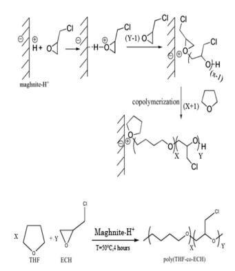
*Figure 8.* Mechanism suggested for the copolymerization of ECH with THF.
