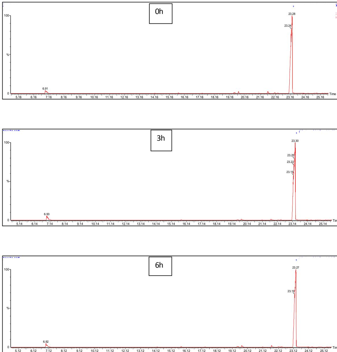
**Figure 5.** Chromatogram of specimens of F45 treated with ultrasound brought into contact with saliva in the presence of agitation and  $\alpha$  amylase.
