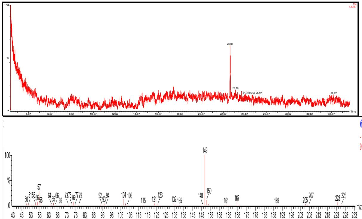
**Figure 4.** Chromatogram and fragmentation ( $m/z = 149$ ) of the DOP internal standard
