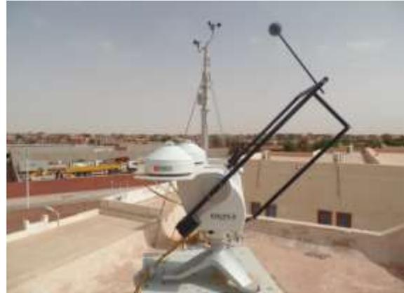
**Figure 1.** Meteorological station installed in URERMS Adrar
