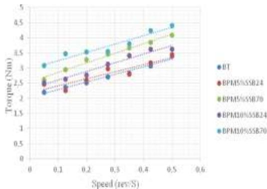
**Figure 3.** Flow Curve of different types of concrete
