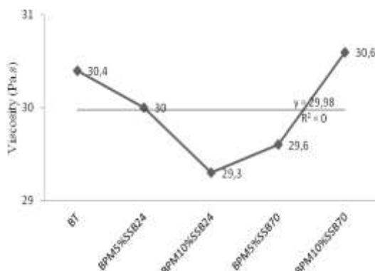
**Figure 4.** Evolution of the viscosity of the different types of concrete
