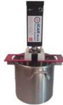
**Figure 2.** The ICAR Rheometer
