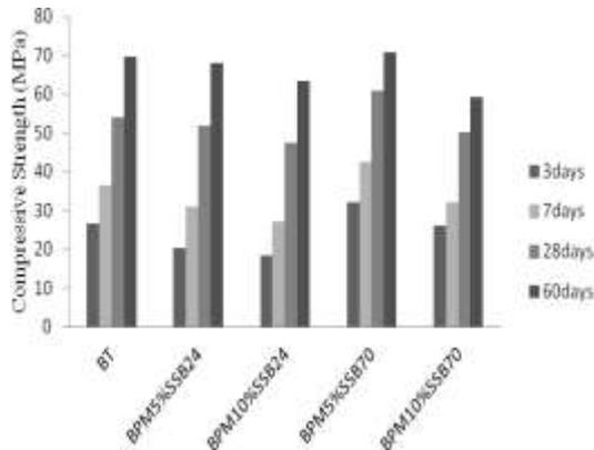
Figure 6. Evolution of the compressive strength of different types of concrete
