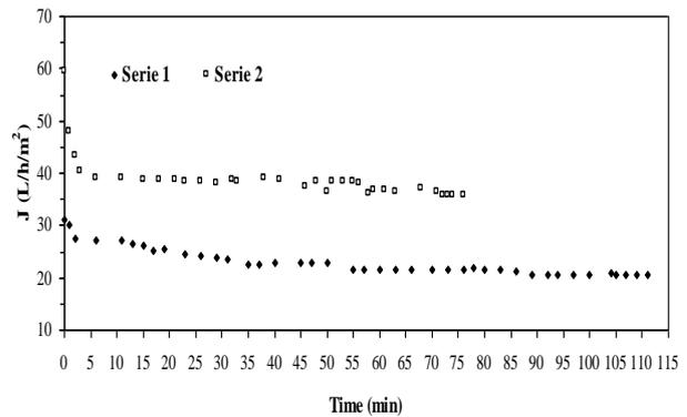
Figure 3. Effect of initial SS concentration on permeate flux during MF of unhairing wastewater (Serie 1: SS = 10.9 g/L; Serie 2: SS = 5.1 g/L).
