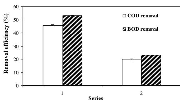
Figure 4. COD concentration and BOD and COD removal efficiency during MF assays (Series 1: SS = 10.9 g/L; Series 2: SS = 5.1 g/L).
