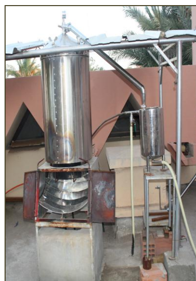
Figure 3: Distillation unit with secondary reflector
