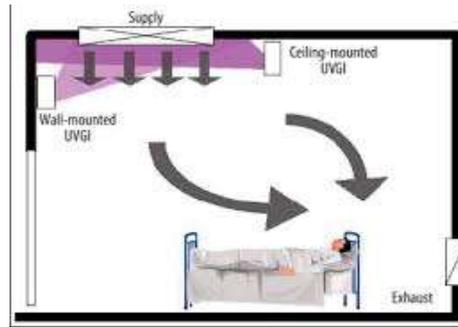
Figure 5. Mixing Ventilation.
