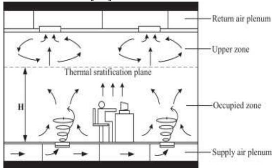
Figure 2. Under floor air UFAD system [28]
