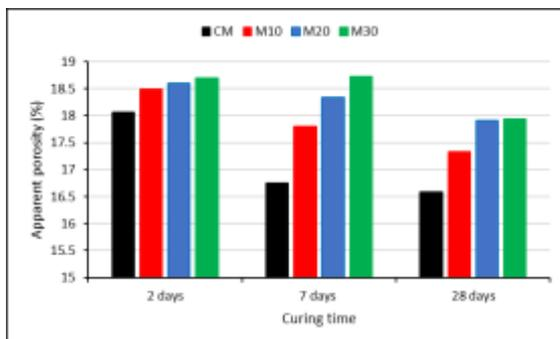
**Figure 6.** Apparent porosity of mortars at different ages.
