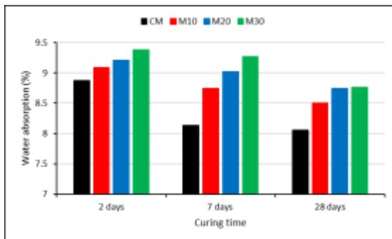
**Figure 5.** Water absorption of mortars at different ages.
