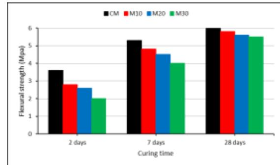
**Figure 2.** Flexural strength of mortars at different ages.
