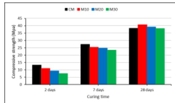
**Figure 3.** Compressive strength of mortars at different ages.
