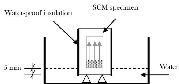
**Figure 4.** Capillary water absorption test for hardened SCM..
