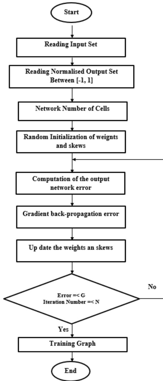
Figure 5. Flowchart of the developed gradient backpropagation algorithm
