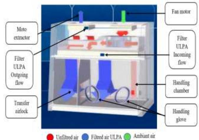
Figure 2. Schematic diagram of the ESCO Isolator
