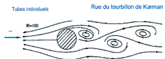
Figure 4. Karman vortex for a bundle and shell heat exchanger for a single tube [31].
