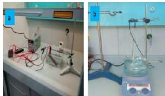
Figure 4. Anodizing processes: (a) Device, (b) Sealing step.
