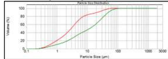
Figure 1. Grain size distribution curves of cement (green) and sewage sludge ash (red).
