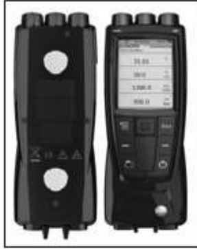
Figure 4. TESTO 480 measuring instrument used in this experiment
